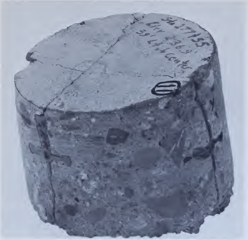
Figure 159.—Intersection of transverse and longitudinal PVC contraction joint-forming waterstops. Upper vertical member on the longitudinal strip is one-half inch longer than that on transverse strip (left). Both strips developed contraction cracks; both joints are sealed; both contraction cracks are continuous across the intersection. PX-D-67427.
